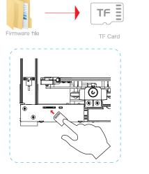
4. Enter the browser to visit https://www.oreality.com/download, download the firmware corresponding to the mainboard according to the model, and write it into the blank memory card. Insert the memory card when the 3D printer is off. CREALITY
